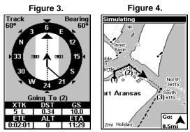
In Fig. 3 the traveler has turned northeast on his new course and is heading straight for Wpt 2, which is 0.28 miles away. Fig. 4 shows route navigation on the Map Page. In this figure, the traveler has reached Wpt 2 and is starting on the leg between Wpts 2 and 3.
